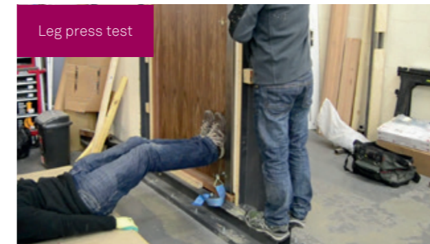
The Leg Press test is an internal test to ensure the doorstop always releases, regardless of pressure on the stop from the inside
