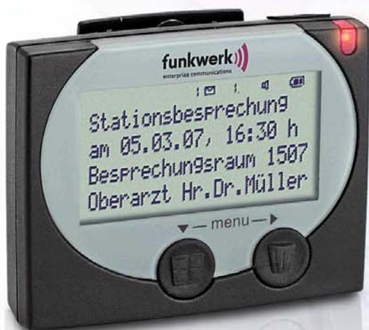
Transmission of manually entered and automatically triggered calls is within a few seconds; the permanent system availability is ensured at any time. The Onsite Communication Processors of the funkwerk OCP series control transmission to specific users or to arbitrarily compiled groups of persons.
