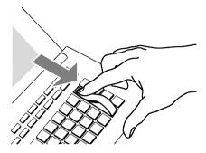
All function keys are pre-assigned with frequently used functions by default. You can insert the relevant legend strips next to the rows of function keys. These can be found on the sheet supplied. If you have changed the assignment of the function keys, you can use the free legend strips on the sheet (for making entries by hand), or use the file included on the CD-ROM (for making entries using a PC).
