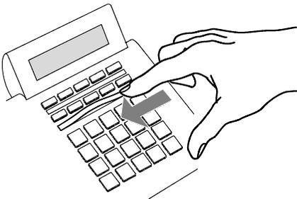
The labelling strips beneath the programmable keys can be filled out and inserted. This allows you to see at a glance which functions are assigned to these keys.
