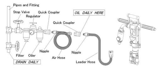
Whether there is any dust, or damage to the air connection portion. Whether the air hose is tight.
