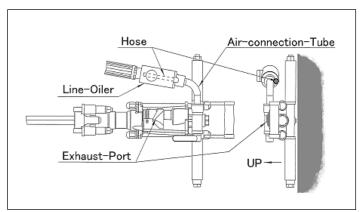
The case that the Hose in the Line-Oiler is set upper than the Exhaust-Port, Oil in the Line-Oiler will leak if the Air hand Hammer is left on the ground with the Exhaust-Port upward.
