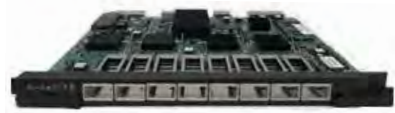
FlexSym Optical Interface Unit (OIU8)
