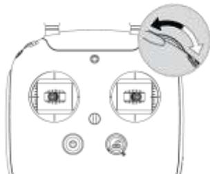
The right wheel sets the camera's exposure value (in automatic mode), or the camera's exposure time (in the manual low ISO mode and manual high ISO mode).
