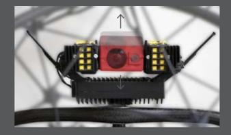
Mounted on a rotatable head the cameras can capture images looking above and below the drone. The full HD camera offers a total field of view of 215° and a horizontal field of view of 130° while the thermal camera offers a total vertical field of view of 42° and a horizontal field of view of 56°.
