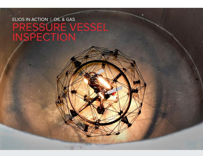
A prevalent tool in energy production and storage are pressure vessels, which hold gases and liquids at high pressures. Vessels are subject to regular inspections, as a ruptured unit can give rise to more fatal risks. Current inspection methods are time consuming and prone to risks; our all-in-one UAV solution Elios can inspect vessels without the risk of injury.
