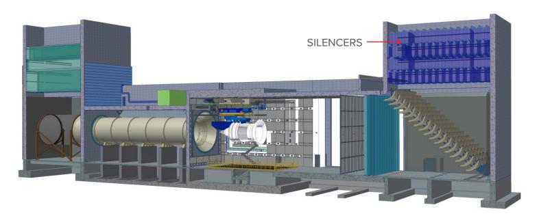
"The presence of control vanes at the bottom of the inlet stack represents a significant obstacle to easily access the silencers."
