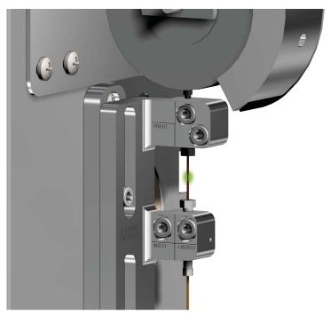
Our innovative FLUX GC×GC flow modulator was designed with one goal in mind—to make GC×GC more routine, accessible, and easier for you. The flow modulator's concept is based on the sound and easily understood principles first articulated by Seeley et al. on diverting flow. This extraordinarily simple design comprising of a cross shape and a sideways T, is not only easy to setup and get started, but its ease-of-use makes it the most cost-effective option for GC×GC analysis.
