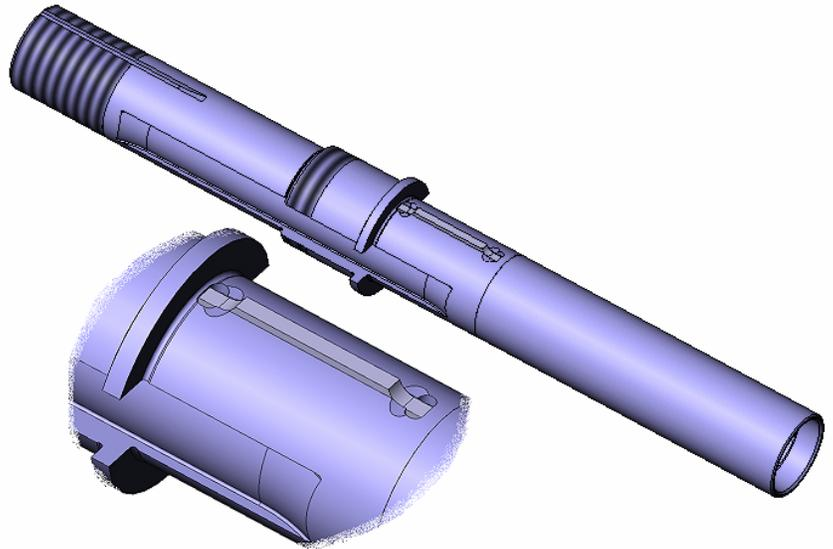
by staking the spindle, actually cold-forming metal from the spindle around the key. We have found this metal-to-metal retention exceeds the strength and durability of all other fastening methods tested, while still offering a full-length, replaceable, cold-formed-hardened key, on a precision bearing diameter. Spindles with shorter, softer, and non-replaceable keys on rough, broached diameters just don't measure up anymore.
