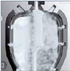
**Sonicated.** Ultrasonic vibrations generate sound-wave energy to create an ultrafine mist
