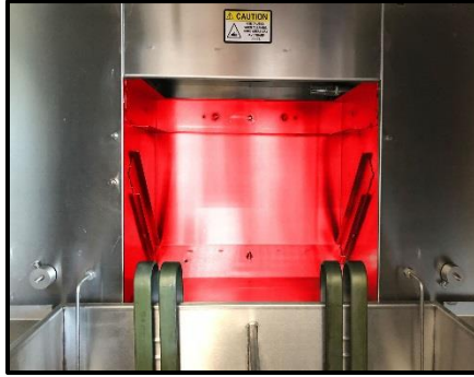
11. Clean / sanitize the ventilation stack and filter tracks.
