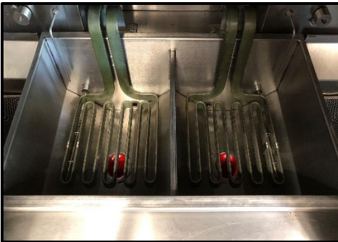
13. Using the long brush the came with the AutoFry, ensure the drain pipes are clear of any blockages.
