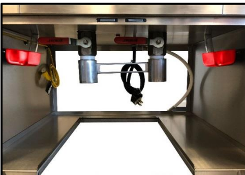
16. Remove and clean / sanitize the grease collector cups located in the lower cabinet.
