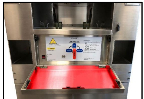
18. Clean / sanitize the OFS valve cover plate.
