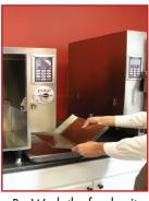
B. Wash the food exit chute with CGR Carbon Grease Remover.
