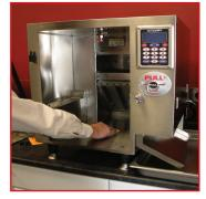
Clean all interior surfaces to bare metal with CGR Carbon Grease Remover and a clean damp cloth.
