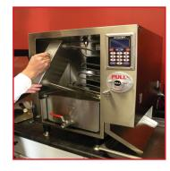
8. Remove the heating element and wipe off any oil with a dry cloth (NEVER SOAK THE HEATING ELEMENT!)
