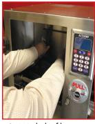
C. Wash the filter cover plate with CGR Carbon Grease Remover.
