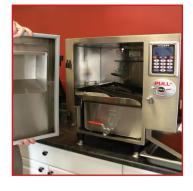
2. Remove the front door of the AutoFry by opening the door and lifting it from the hinges.
