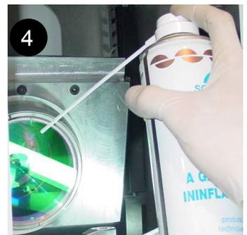
7. Soak slightly an optical paper towel in optical cleaning fluid.
