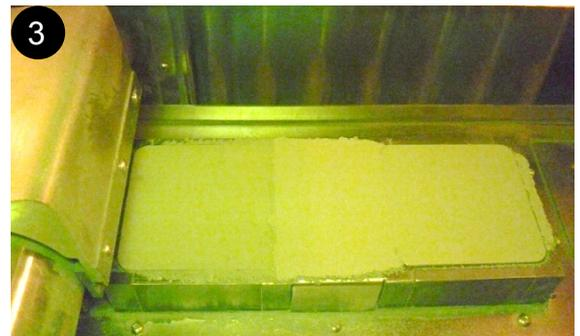
3. If the powder bed is not properly completed, re-run the powder bed cycle. Proceed the next section only if the powder bed cycle is properly completed.
