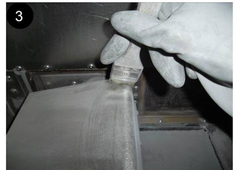
4. Move the carriage up to the sintering piston, then clean the left side of the manufacturing chamber (4), sweeping the powder toward the collecting cans.
