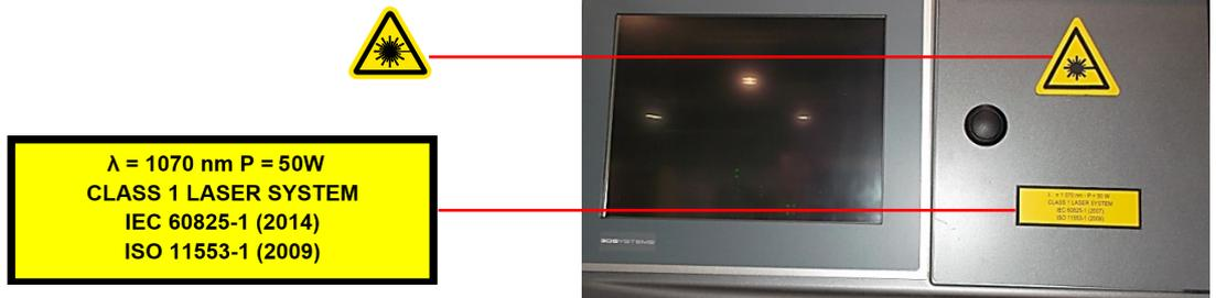
**Laser Safety Labels - Located on the scanner head**
