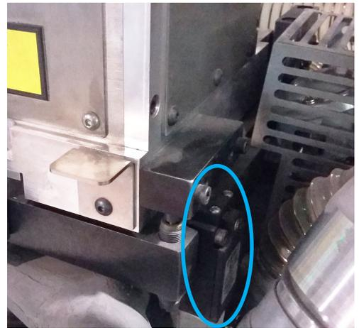
**D** Safety interlock switch on the airlock door
