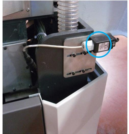
**C** Safety interlock switch on the scanner head
