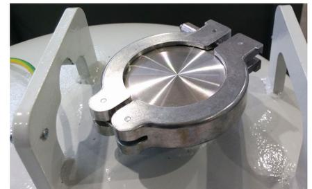
Step c : clamp tightening
