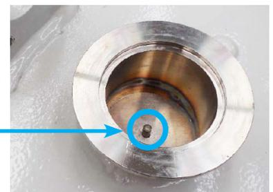
The external pneumatic valve is placed directly on top of the centering ring with stand-off and pressed down until the flanges meet. This creates the seal between the two parts and the centering ring with stand-off holds the spring-loaded valve open for normal operation. The connection is secured with a clamp.
