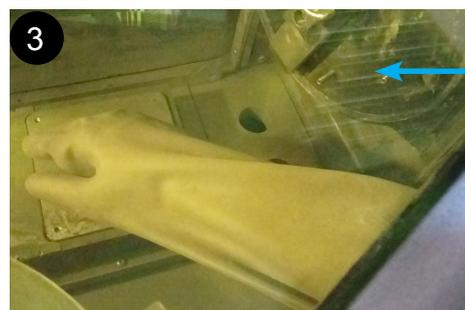
13. Remove the paper towel (used to protect the sintering plate) from the airlock.
