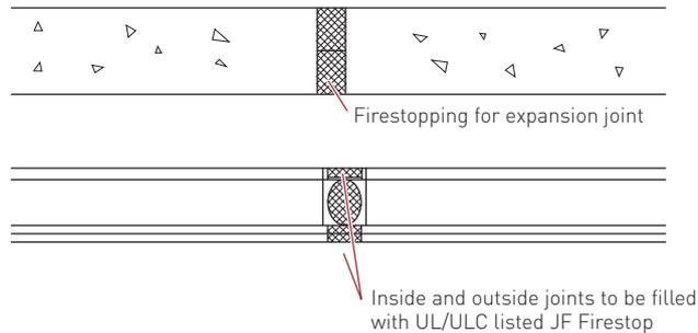
**Fig. 4 Protection of expansion, and inside and outside joints**
