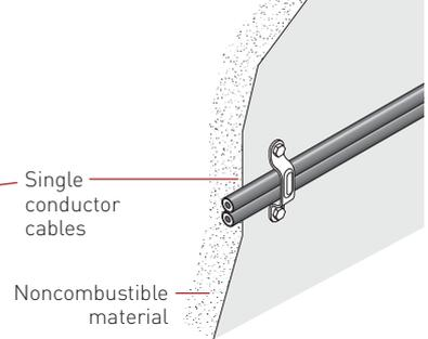
**Fig. 6 MI cable installed on noncombustible surface**
