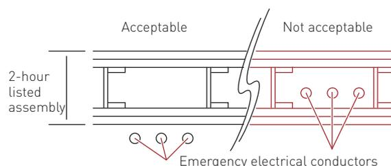
Fig. 3 Protection of emergency conductors using drywall/gypsum
