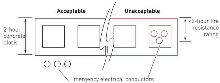
**Fig. 5 Protection of emergency conductors using concrete block**
