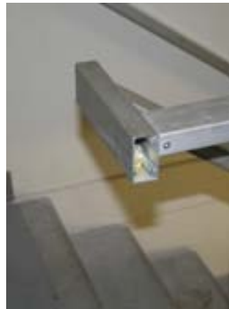
Side rail is damaged, limiting safe use
