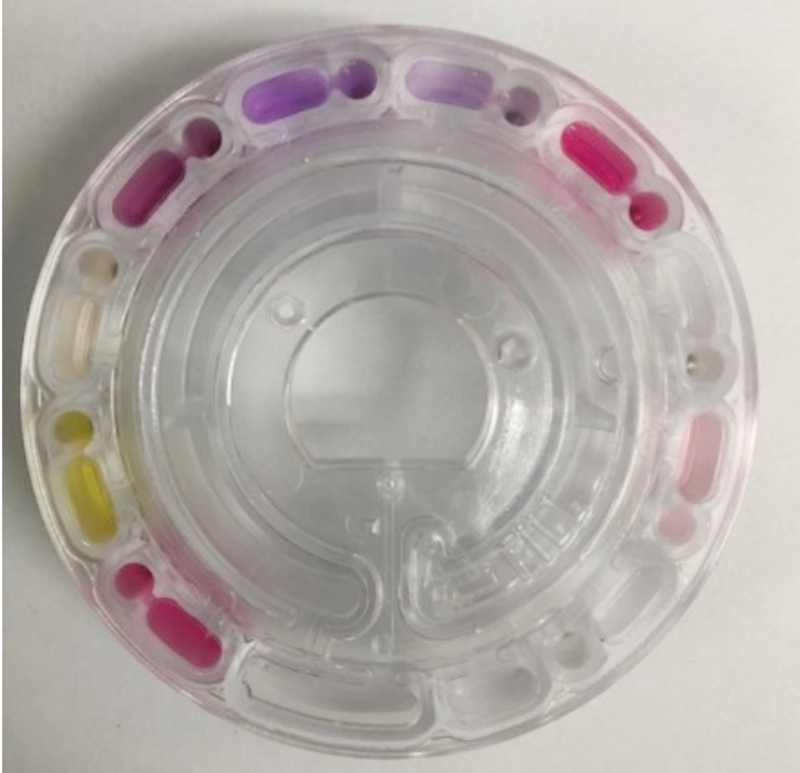
This is an example of a cooling tower disk after spin out, the colors in the wells determine the readings.
