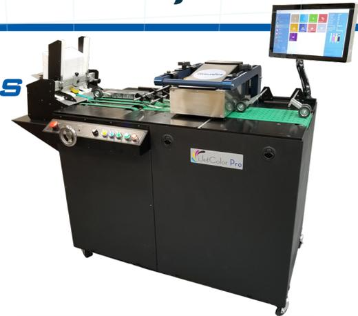
The iJetColor Pro is a high-speed, light industrial envelope and packaging printer that can print full color. With the capability to print short-run, full-bleed variable data jobs or odd-sized materials, the iJetColor Pro is your workhorse to produce cost-effective, personalized materials easily and profitably.
