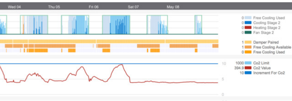
Figure 1: System performance overview. Light blue areas indicate when the system is using outside air for free cooling.
