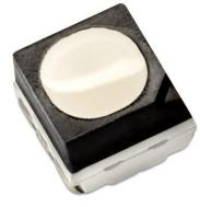
Module 0.5W outperforms all competitors, producing red light of 1,000 mcd, green light of 2,300 mcd and blue light of 500 mcd at 20 mA drive current (typical Vf of 2,1, 2.8 and 3.0V, respectively).
