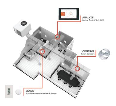
Sensors collect data from each room every minute. Each night, cloud computing algorithms analyze thousands of data points, including the weather forecast, enabling the system to predict future conditions. A new set of instructions are then sent to the Central Control Unit and the dampers are modulated a few degrees at a time to achieve the perfect balance. The system also factors in real time events, such as room occupancy, to make instant adjustments to the plan as needed.
