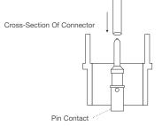
**Step 3:** This step varies on the connector series. On the mating face of the connector, insert the tool over the pin contact or into the socket contact until the tool bottoms. Apply slow, continuous pressure to push the contact out of the rear of the connector. When the shoulder of the tool "thunks" against the insulator, the contact is extracted.
