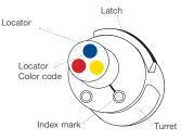
**Step 3:** Select the proper locator position for your contact by rotating the locator until the proper color is aligned with the index mark. Push the locator back down until it snaps into position.
