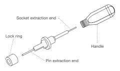
**Step 2:** Use the proper extraction tool (based on connector series and contact size). The extraction tool can be used for both pin and socket contacts by removing the shaft from the handle and reversing it for pin or socket extraction (not applicable to all types).
