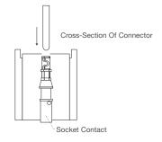
**Step 4:** Carefully remove the extraction tool from the connector to avoid damage to the insulator.
