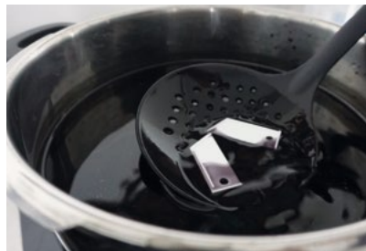
Figure 2-4: Pouring textile dye into the water, putting the parts in the pot, drying the parts
