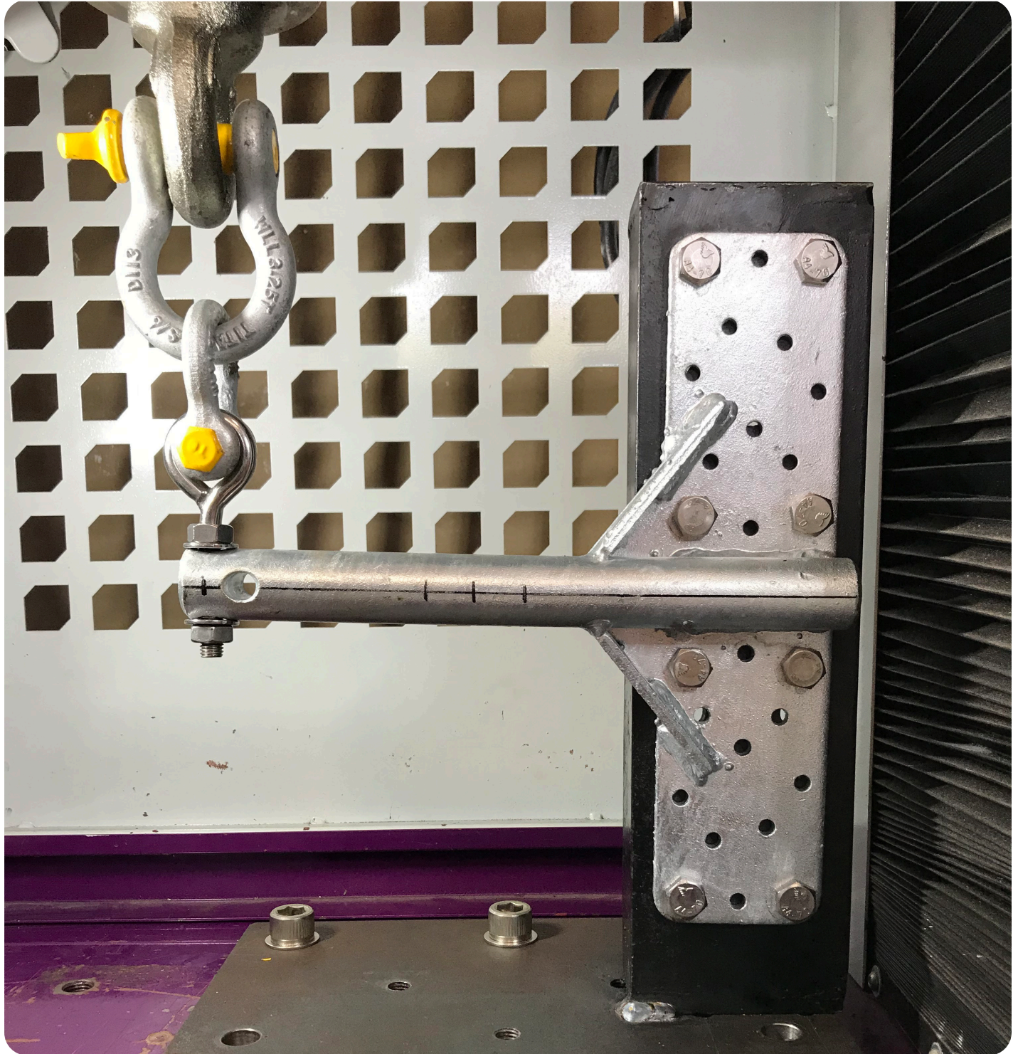
Picture 3 - Taken with 1250kgf load applied. Rafter Bracket returns to original shape when load is removed. No permanent deformation whatsoever.
