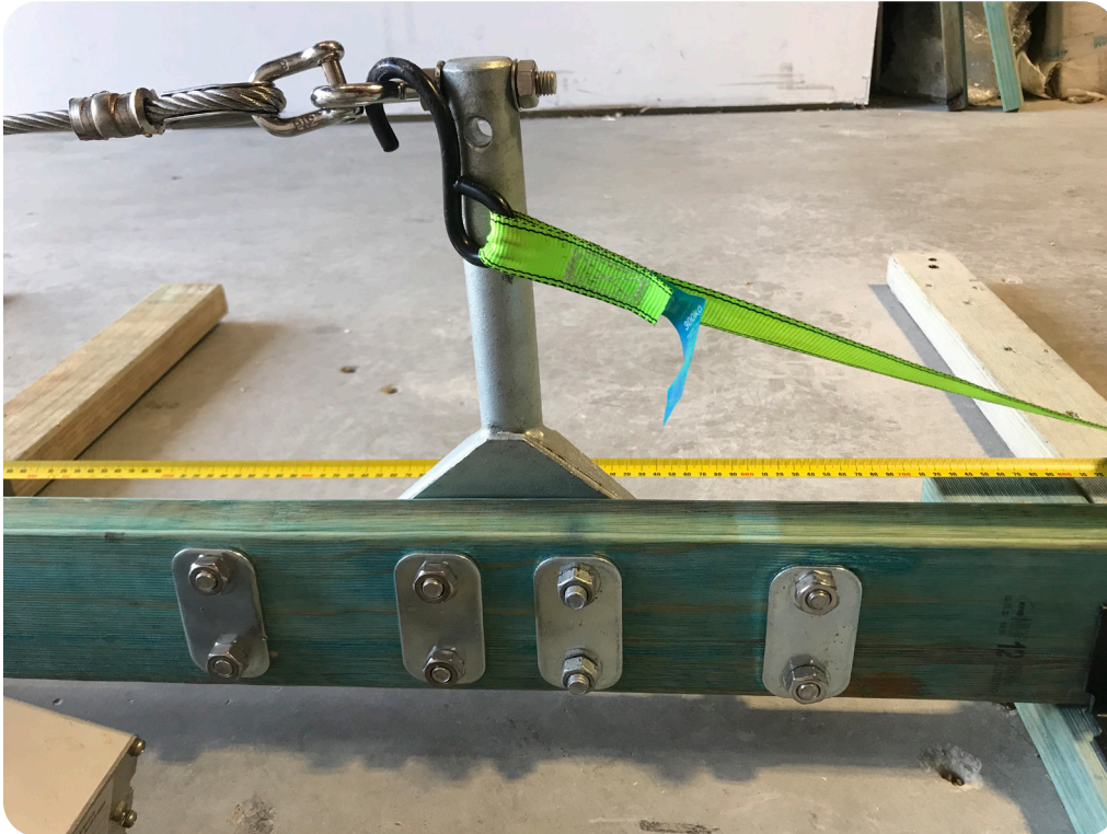
Picture 1 - Test shown above has Rafter Bracket fixed to 90 x 35mm structural pine MGP12. Load held static at 1250kgs for 7 days without failure.
