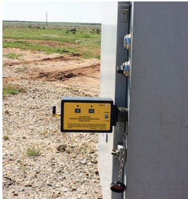
Fig. 13. Echometer’s new wireless power measurement system.
