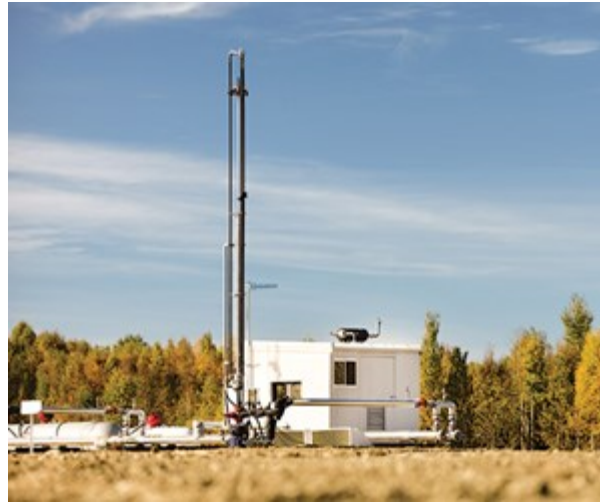
Fig. 5. The Zedi SilverJack linear lift system.
