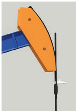
Fig. 12. Bright's Wireless Load Cell mounted at the head of a beam/rod pump.
