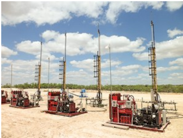
Fig. 3. Several CAMLIFT 40-192 linear lift systems employing Cameron's new counterbalance system.
