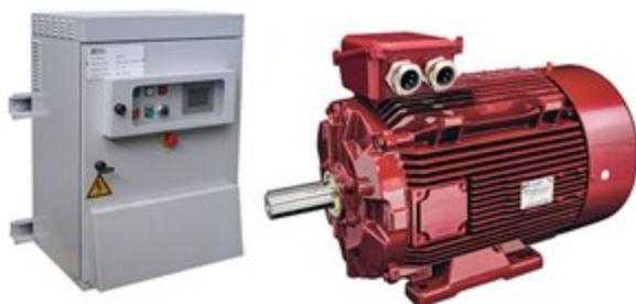
Fig. 10. Emerson's Powerdrive FX four-quadrant VSD (left), and their LSRPM synchronous magnet-type motor (right) enhance rod pump operations.
