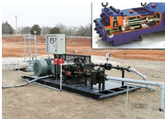
Fig. 9. Ultra-Flo system with a T-Series diaphragm pump (inset).
