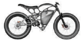
The Light Rider's frame, which weighs just 13 pounds, is made of aluminum particles melted together by a laser. Only 50 of the electric motorcycles will be produced.
