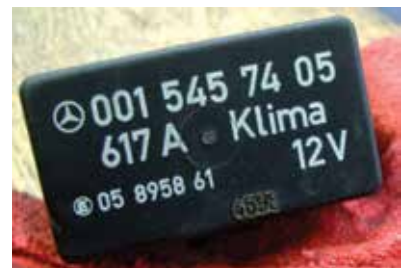
Since Mercedes-Benz vehicles last longer than other makes, you might still be seeing the KLIMA relay in your shop. While it’s more complex than a basic relay, it can still be tested directly.
