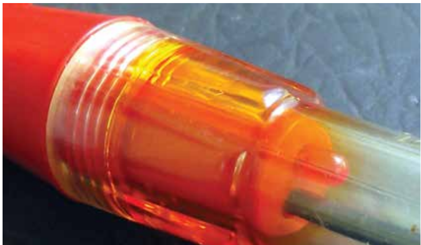
...always use the LED type as the old-fashioned incandescent-bulb variety can draw enough current to damage electronics.
