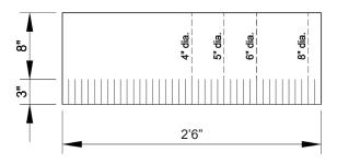
For other sized penetrations or if the diameter is not known, simply wrap the skirt around the pipe allowing for minimum 1 in (25 mm) vertical overlap, mark the skirt and then cut accordingly.
