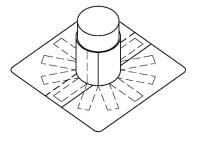
For top applied flashings, remove masking tape while resin is wet when used.
