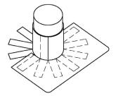
Then immediately follow with the second target piece to fit tightly around the pipe penetration, overlapping the underlaying target piece 2 in (51 mm) minimum, using a catalyzed basecoat and topcoat of ALSAN RS resin.
