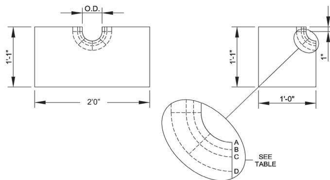
Additional equidistant relief cuts may be made as required to assure the targets lay flat around the penetrations. For other penetrations or if the diameter is not known, simply drape the target around the pipe, mark and then cut accordingly.
