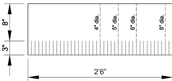
For other sized penetrations or if the diameter is not known, simply wrap the skirt around the pipe allowing for minimum 1 in (25 mm) vertical overlap, mark the skirt and then cut accordingly.
