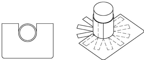
Then immediately follow with the second target piece to fit tightly around the pipe penetration, overlapping the underlaying target piece 2 in (51 mm) minimum, using a catalyzed basecoat and topcoat of ALSAN RS resin.
