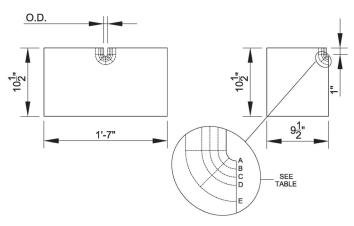
Additional relief cuts may be made as required. For other penetrations or if the diameter is not known, simply drape the target around the pipe, mark and then cut accordingly.
