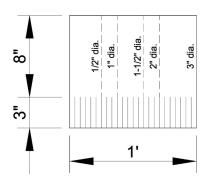
For other sized pipes or if the diameter is not known, simply wrap the skirt around the pipe allowing for minimum 1 in (25 mm) vertical overlap, mark the skirt and then cut accordingly.
