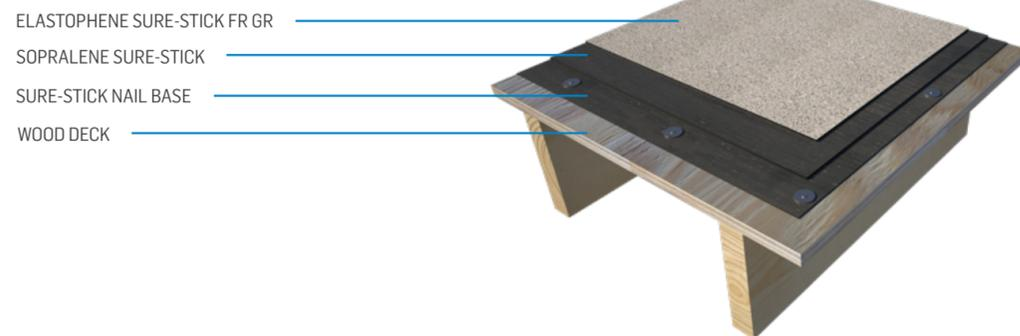
\* SOPRALENE or ELASTOPHENE SURE-STICK base/interplys may be used in either assembly based on design requirements.
