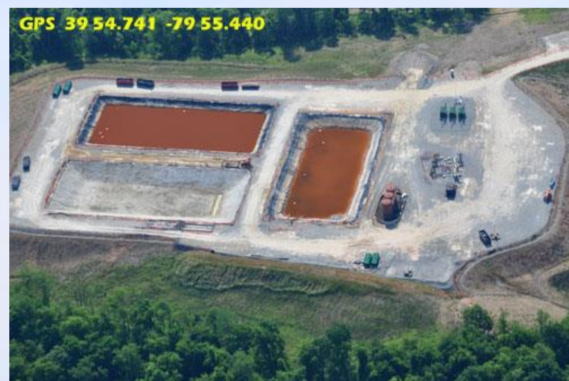
Much of the natural gas burned by power plants in ISO New England comes from Hydraulic Fracking, which uses open air water impoundments (shown above) to store toxic wastewater.
