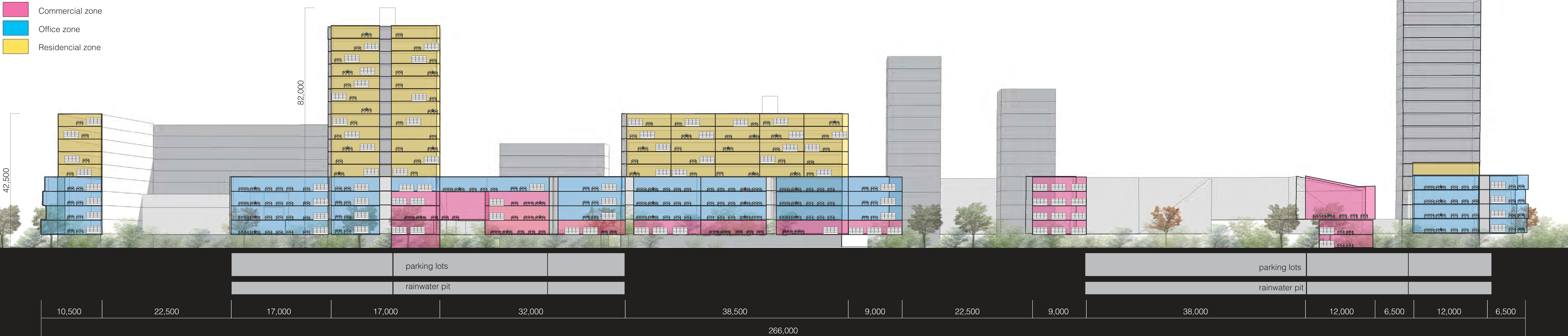
Section A-A' scale=1:500 Set atrium and courtyards to maximize the horizontal space incorporating natural sense of space.
