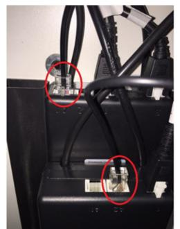
6. Switch the port from A1 to A2 or vice versa for the hand control extension cables in the black control box - for the front or the rear table that is having the issue.
