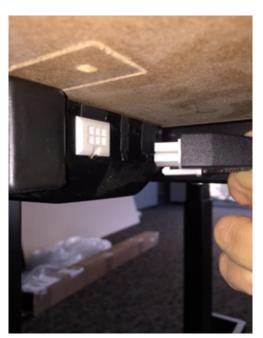
3. If this does not solve the problem, check that leg extension cables are plugged in fully into the leg ports.
