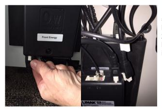
5. Check that the leg extension cables are plugged into the control boxes tightly. There is a front control box with legs going into Port 2 on the bottom and Port 1 on the top. The rear control box could have the same ports as the front OR an additional leg cable going into Port 3 on the top – if the rear table has 3 legs).
