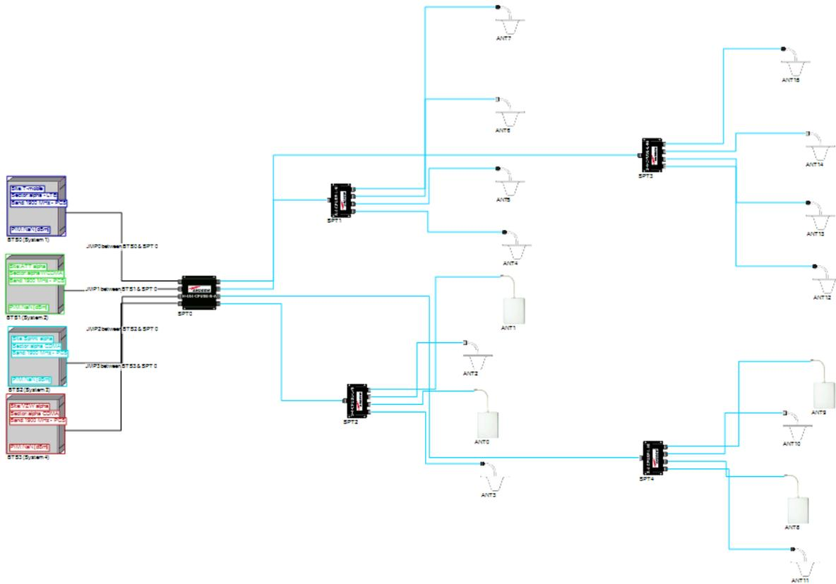
Figure 5: Passive DAS architecture
