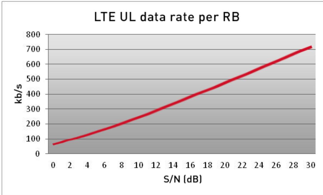
Figure 4: Uplink LTE data rate per Resource Block
