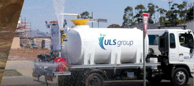
Filling up a bowl (tree watering) with the old truck took roughly 25 seconds, now with the TTI Cascade - **it takes less than 10 seconds.**
