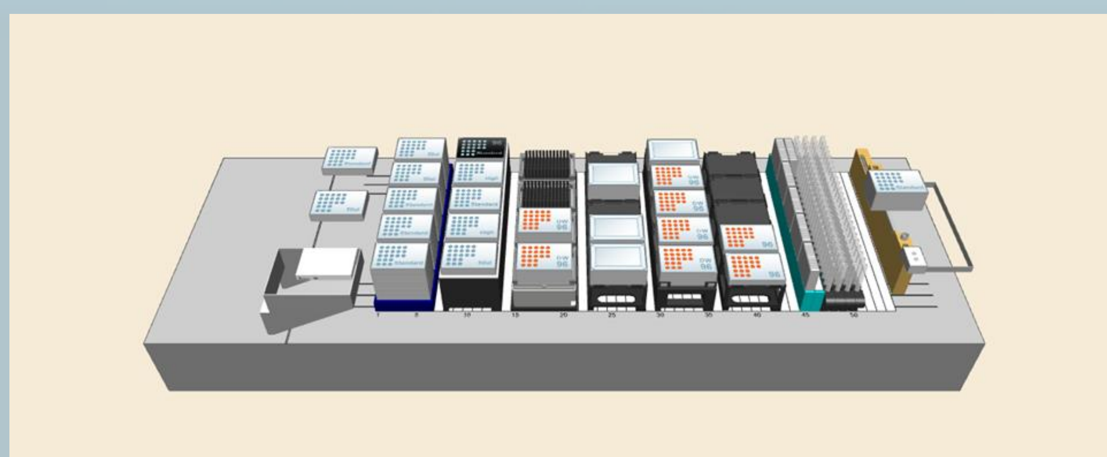
Figure 3: Hamilton Microlab STAR deck configuration for microsome clearance assay
