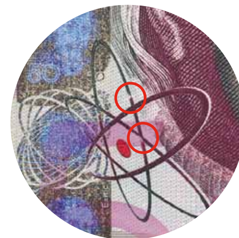
BANKNOTE REJECTED DUE TO THE LINE BREAKS IN THE ORBITAL RINGS
