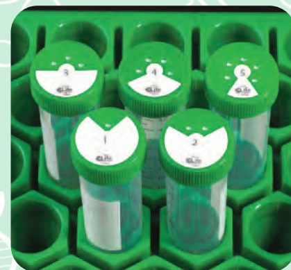
Vent control labels for 50mL Bio-Reaction Tube Caps cover 1 to 5 of the cap vent openings to control the amount of gas exchange
