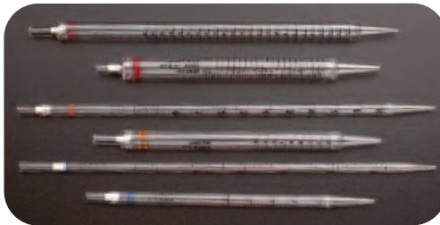
Short vs. standard length pipet comparison
