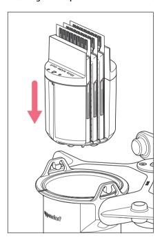
Insert the loaded adapter in the round bucket and make sure that the arrow on the adapter is aligned with the marking on the bucket. Make sure that the imprint "this side out" on the adapter points outward.
