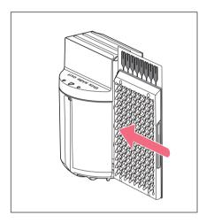
▶ Insert the 3 plates with the filler flap pointing upward (see figure). The plates must be seated completely inside the adapter.
