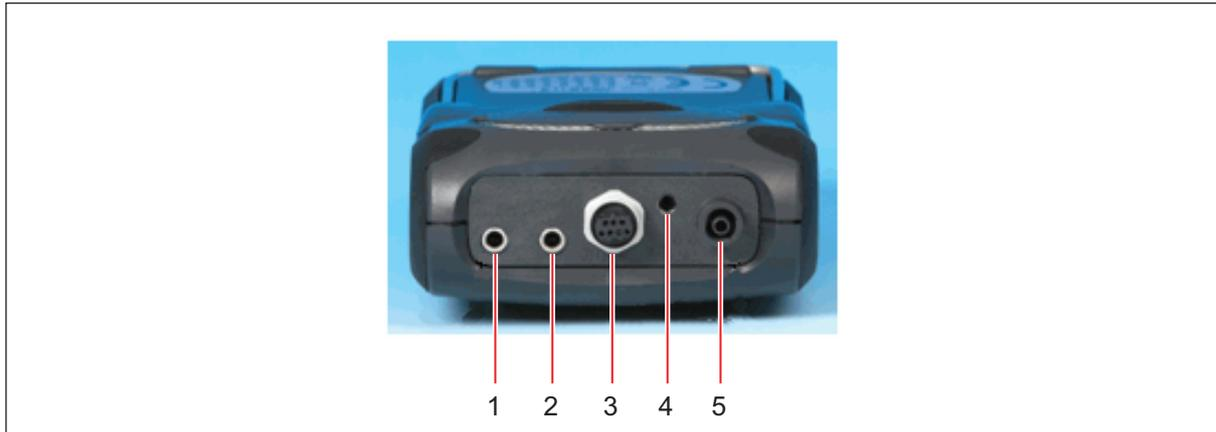
Fig. 4-3: Connection points - Top view
