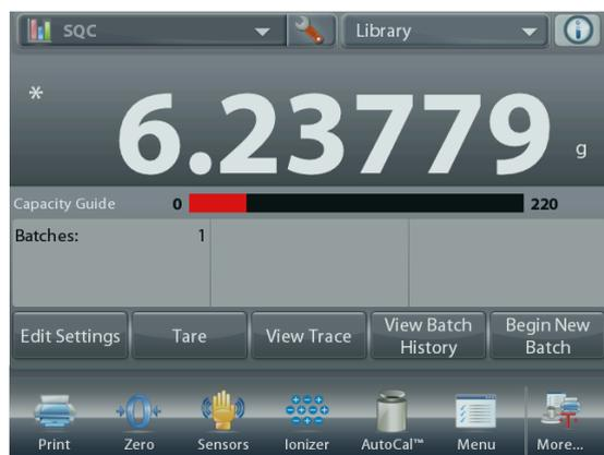
To view the Process results graphically (batch comparison), press the **View Trace** button.
