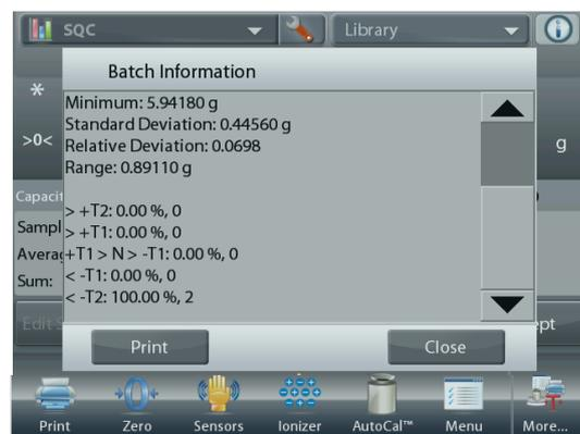
To view the process results of this batch (and any other saved batch), press the **View Batch History** button.
