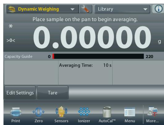
After the cycle ends, remove the specimen and the balance returns to the Home screen automatically (after a 10-second delay).
