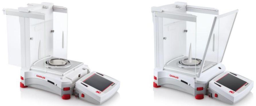
Press button to separate Terminal from Base. Seat panel's hooked ends in base. Swing panel to vertical position.
