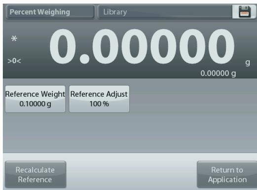
To establish a new Reference weight value, touch the **Recalculate Reference** button.
