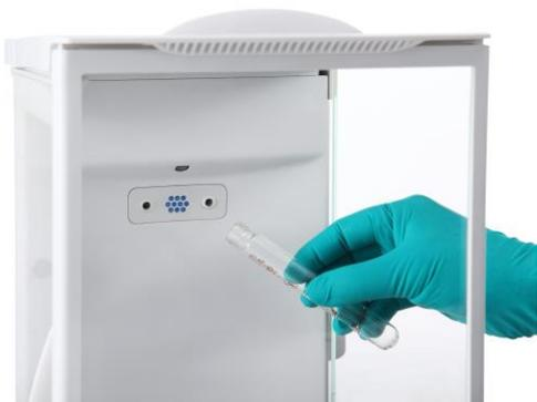
The Ionizer generates bipolar ions continuously by DC corona discharge separately from positive and negative discharge electrodes and directs the ionized air onto the charged body to eliminate static electricity. The generated ions are well-balanced in polarity and can eliminate static electricity regardless of the polarity of the charged body.
