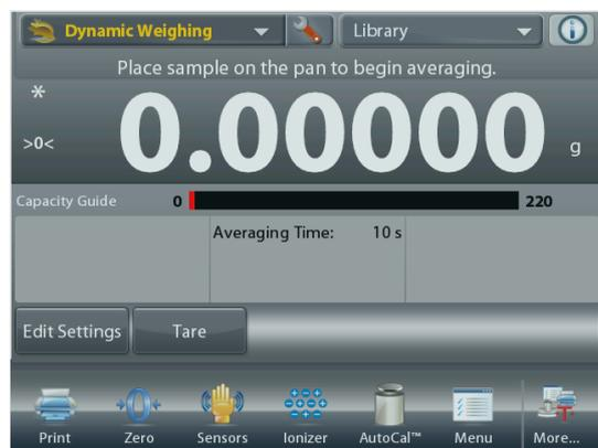
Place specimen on the Pan. The cycle starts automatically.
