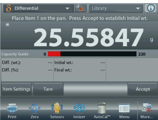
After **Accept** is pressed, the difference between initial and final weights appears in the Reference Fields.
