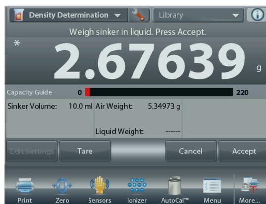
Once the necessary weights have been determined, the density of the Liquid sample is displayed in **g/cm<sup>3</sup>** (along with the weight in air, weight in water) on the Application screen.
