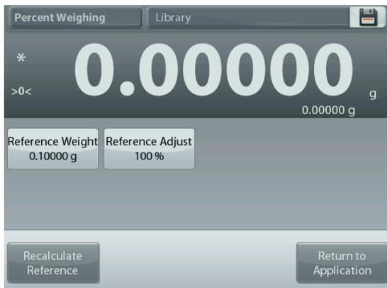
The current Reference weight value is shown on the Settings screen. To adjust the Reference weight directly, touch the **Reference** button.
