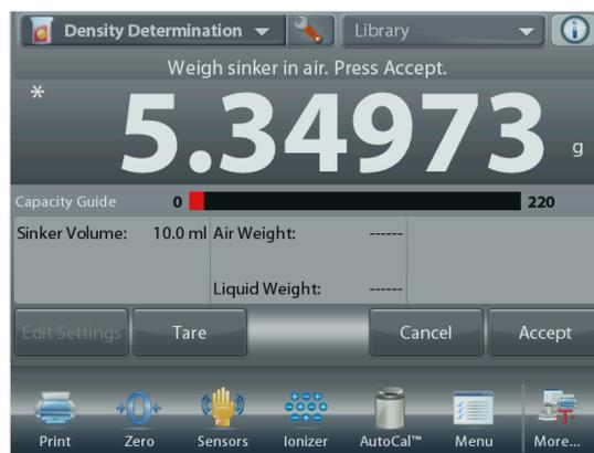
**Step 2 of 2 – Weigh the Sinker Submerged in the Test Liquid.**
