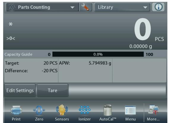
The default (or last) Average Piece Weight (APW) is displayed. Place objects on the pan to display the Fill Status.
