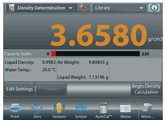
Once the necessary weights have been determined, the density of the sample is displayed in **g/cm<sup>3</sup>** (along with the weight in air, weight in water) on the Application screen.
