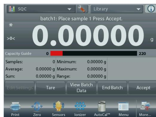
At any time, press **End Batch** to see the Individual results screen, showing results for the current Batch.
