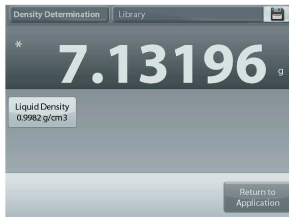
Measure the actual liquid density of the Density setup and enter it.
