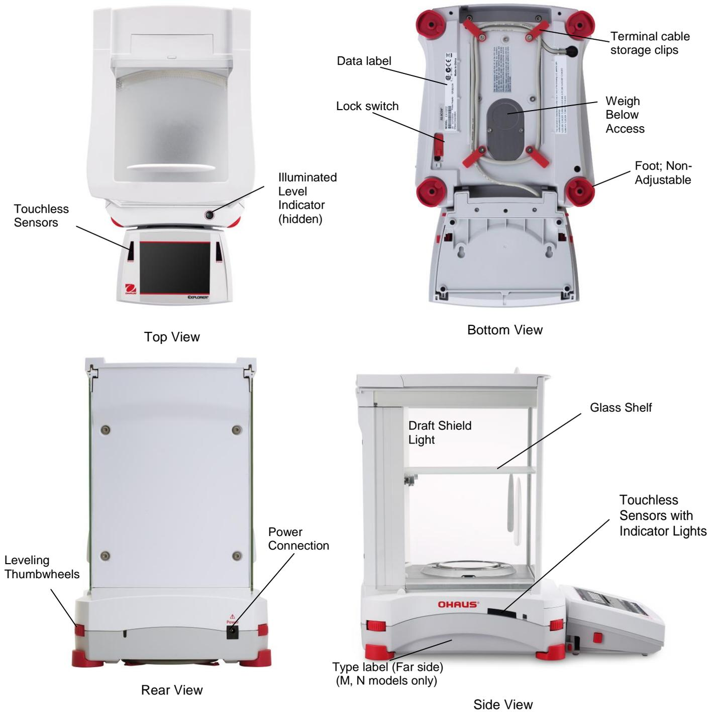
Figure 3-1. Explorer Semi-Micro Balance
