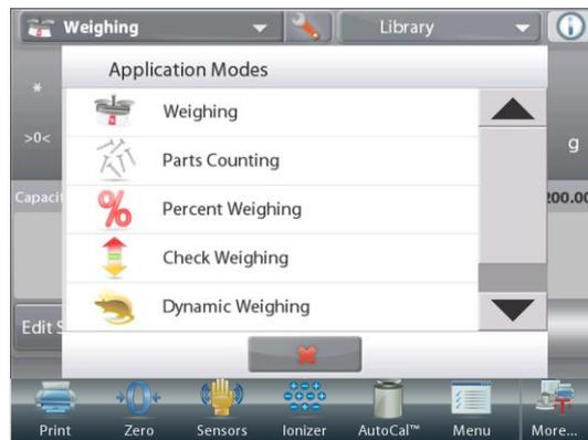
Note: If an application mode does not appear in the list of available Applications it must be **enabled** in the User Menu: touch **Menu**, then select **Application Modes**. The full list of modes appears. Touch the one you want to enable. Then touch **Enabled** in the setup menu for that application mode – Percent Weighing in the example below. Each enabled mode appears in the **Applications** menu.
