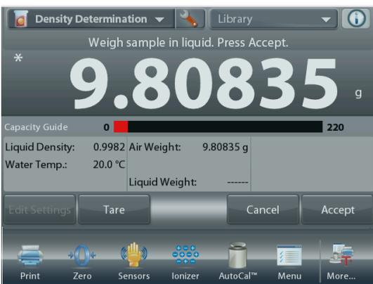
**Step 2 of 2 – Weigh the Sample Submerged in the Liquid.**
