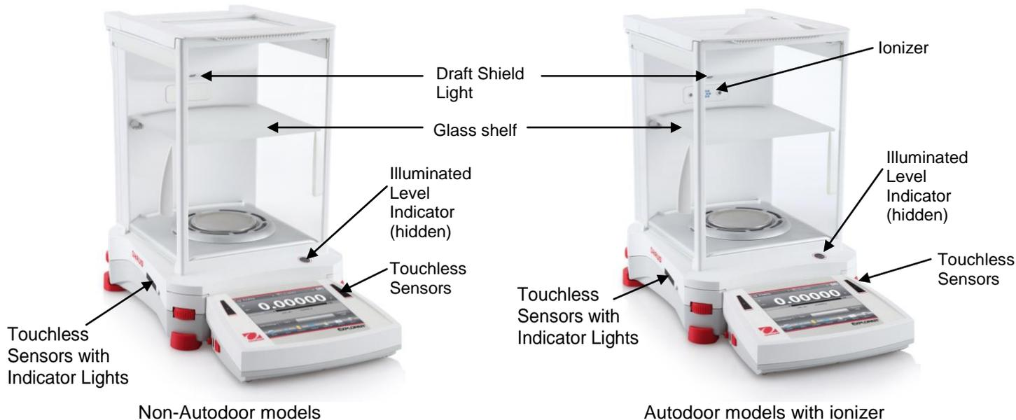
Figure 3-3. Non-Autodoor and Autodoor models with ionizer
