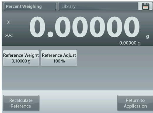
A numeric input window appears. Key in the desired Reference Weight Adjustment, then press ✓.
