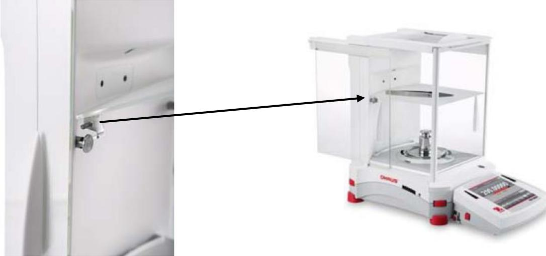
Align and press down the shelf on the two supporting pegs.
