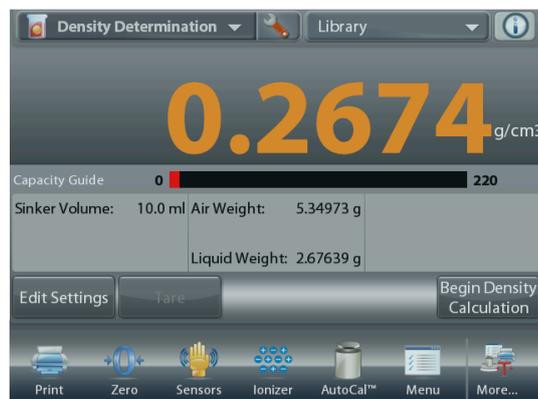
4.10.6 Measuring the Density of Porous Material Using Oil
