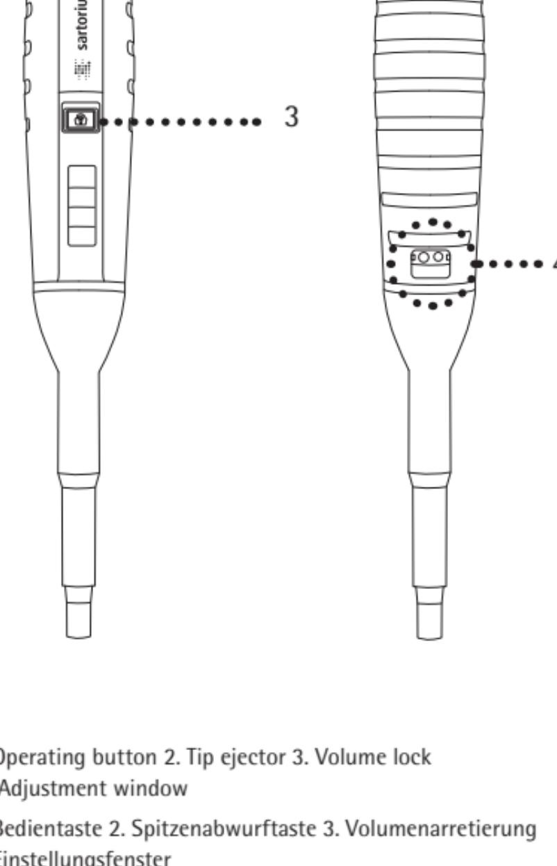
1. Operating button 2. Tip ejector 3. Volume lock
