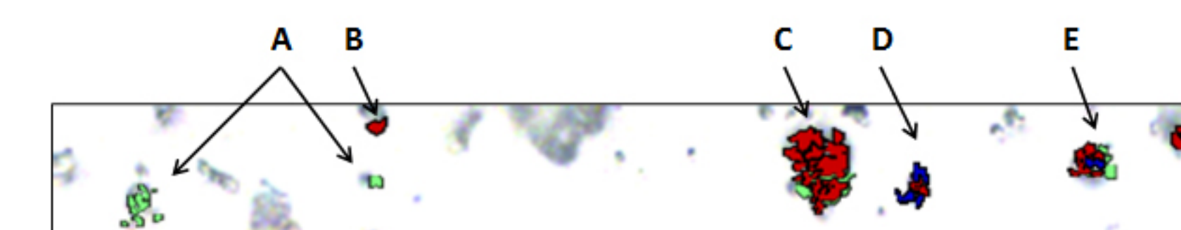
Figure 3. Representative fusion BFR/RCI image of free standing and agglomerated particles in a DPI formulation where Fluticasone is false-colored in Green, Salmeterol is false-colored in Blue and Lactose is false-colored in Red.
