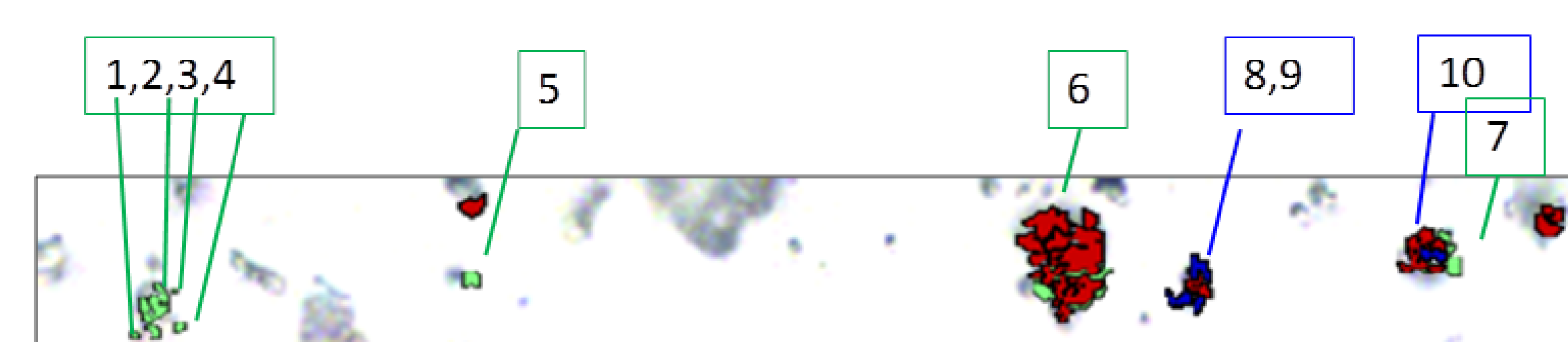
FIGURE 1 Representative fusion image of free standing Fluticasone propionate particles versus bound to carrier particles in Seretide® where Fluticasone Propionate is false-colored in Green; Lactose is false-colored in Red; Salmeterol Xinafoate is false-colored in Blue.
