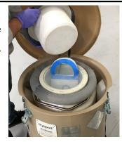
Install the Vapor Plug and allow it to seat down completely
