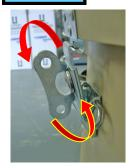
Unlock latch by turning the key to the left.
