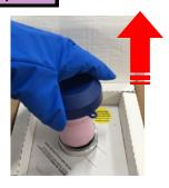
Remove the dry shipper vapor plug.
