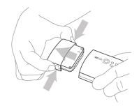
Detach Control Module and attach it to a Mini USB Charger for 6 hours.
