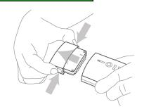
Detach Control Module and reattach it to the a Fresh Battery Pack to the new battery pack
