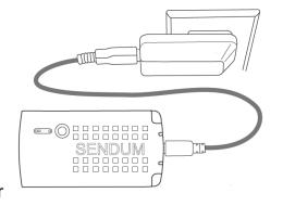
Reattach Control Module to Charged Battery Pack
